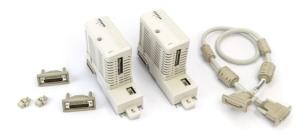
The BC810 unit consists of two basic parts: baseplate (TP857) and power supply/logic board. The baseplate is where the connectors to CEX-Bus and the external power reside. It is grounded to the DIN-rail through metal parts of the housing. The board also carries the external power voting diode and fuse. The power supply and logic board contain the +3.3 V converter, logic, drivers for CEX-Bus interconnection, and the connector for the interconnection cable.
