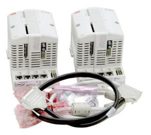
The CPU board contains the microprocessor and RAM memory, a real-time clock, LED indicators, INIT push button, and a CompactFlash interface.
